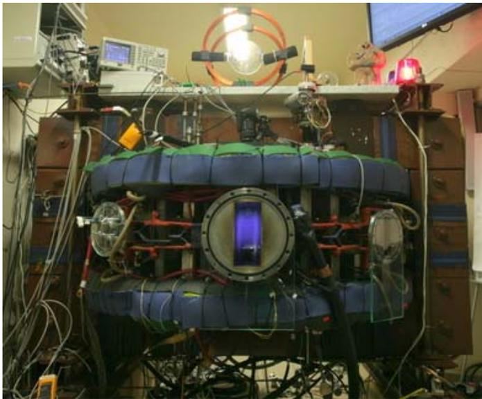
*Fig. 1: Golem Tokamak in action. Photo: courtesy The Golem Team*
